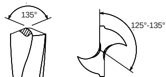
Heavy Duty Notched Point Point Entaille à grand rendement Eingekerbte Spitze Schwereinsatz Punta ranurada para uso intensivo Усиленная вершина Notched Point
